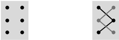
Fig. 2: Two controller layouts are shown (controllers are shown as black dots). Left: Single leg - one agent controls each leg, imposed to all legs. Right: Tripod - control for two legs is learned, imposed to groups of three legs each.
