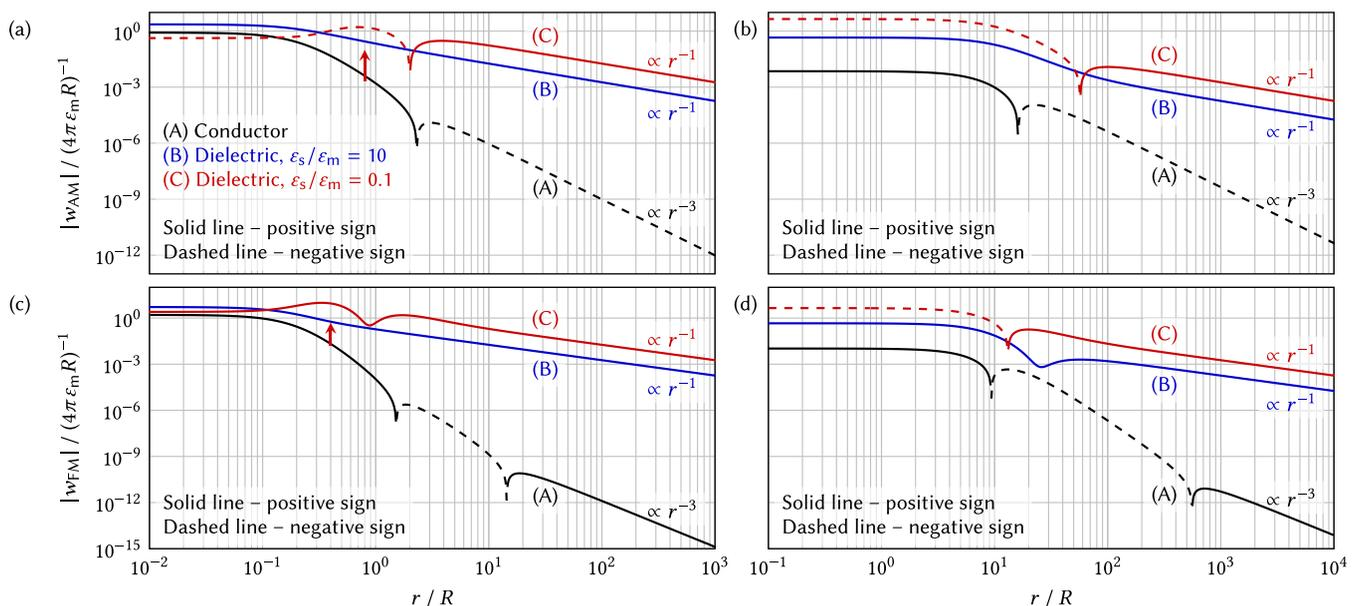
FIG. 5. Profile of the weight functions as a function of the lateral distance  $r$  for charges at a fixed height of  $z = R/100$  above the sample. The AM-KPFM weight function is shown in (a) and (b), while the FM-KPFM weight function is shown in (c) and (d). In the left column [(a) and (c)], the tip-sample distance is  $z_{ts} = R/40$  and in the right column [(b) and (d)] the tip-sample distance is  $z_{ts} = 10R$ .
