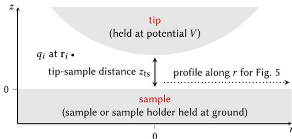
FIG. 1. Schematic view (not to scale) of the considered model for the probe tip and the flat sample. The spherical tip (which is not shown completely) is laterally centered at  $r=0$  and at a distance of  $z_{\text{ts}}$  above the sample surface, which is located at  $z=0$ . A set of point charges  $\{q_i\}$  at position  $\{\mathbf{r}_i\}$  can be placed in the tip-sample system.
