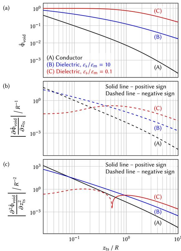
FIG. 4. (a) Normalized electrostatic potential at  $r=0$  and  $z=R/100$  as a function of the tip-sample distance  $z_{ts}$  for the void tip-sample system. The first and second derivative with respect to the tip-sample distance  $z_{ts}$  (relevant for AM- and FM-KPFM) is shown in (b) and (c), respectively.
