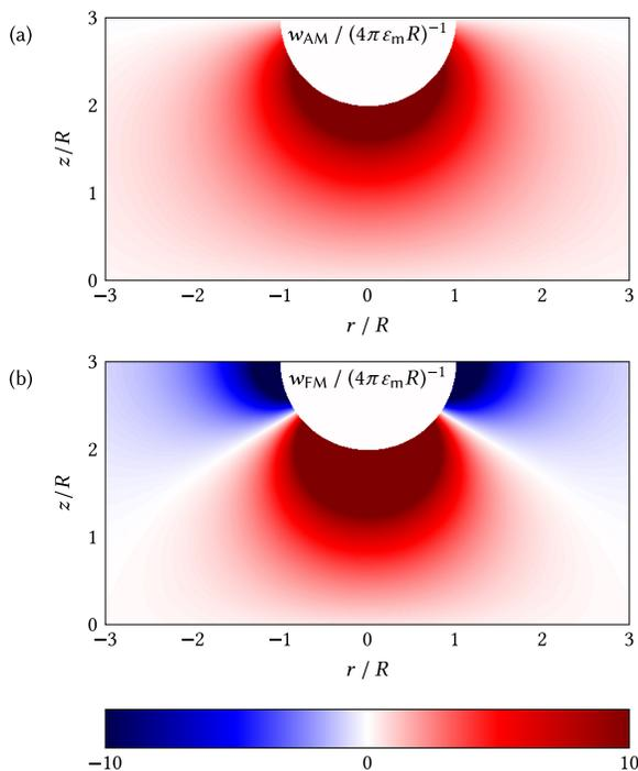
FIG. 2. Weight functions for case (B) with a tip-sample distance of  $z_{\text{ts}} = 2R$ . The AM-KPFM weight function is shown in (a) and the FM-KPFM weight function in (b). The sample surface is located at  $z = 0$ . The color bar shown below applies for both plots.
