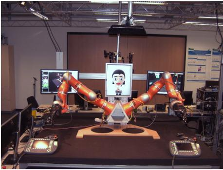
Fig. 1. The FAMULA platform: A bimanual robotic platform supporting the investigation and development of approaches by which a cognitive system can familiarize itself with new objects and concepts through the interplay of manual action and language (<https://www.cit-ec.de/en/deep-familiarization-and-learning>).
