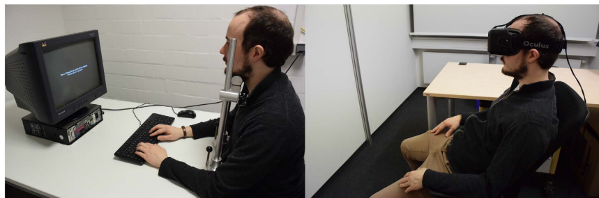
Figure 2. Assessment setups. A participant sitting in front of a standard CRT with head position fixed by a chin rest (left) and wearing the Oculus Rift virtual reality device (right).
