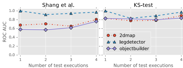
Fig. 5. Influence of the number of test executions on the two most promising detection methods. For Shang et al. the max aggregation method was used and for the KS-test the mean of all counter scores.
