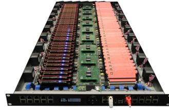
Figure 8: Example of a RECS®|Box system equipped with 72 ARM compute boards
