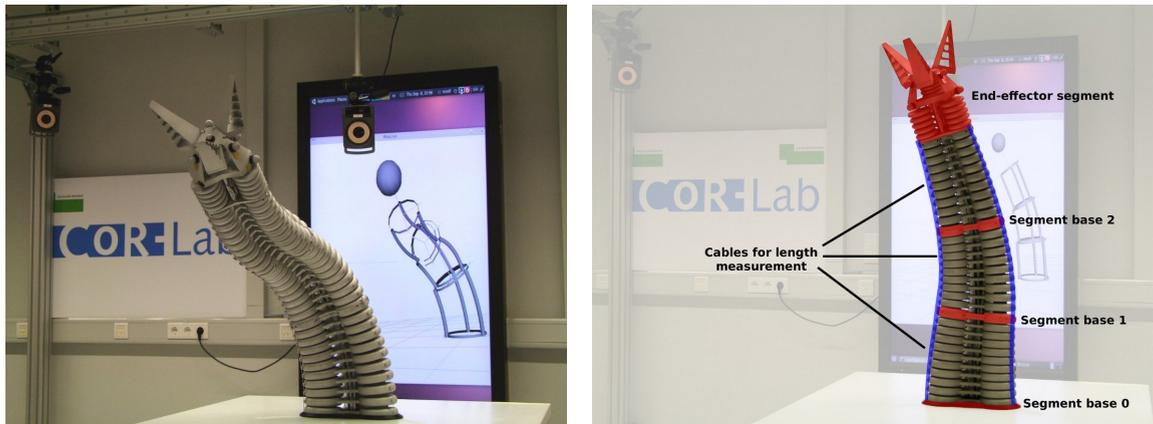
Fig. 1. Left: The Bionic Handling Assistant (BHA) is a pneumatically actuated, soft robot trunk manufactured by Festo. Right: The BHA comprises three main segments with three air chambers each and a gripper segment. The length expansion of air chambers is measured by cables running along the outer hull of each chamber.
