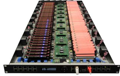
**Figure 2: Example of a RCU, equipped with 72 ARM compute boards**
