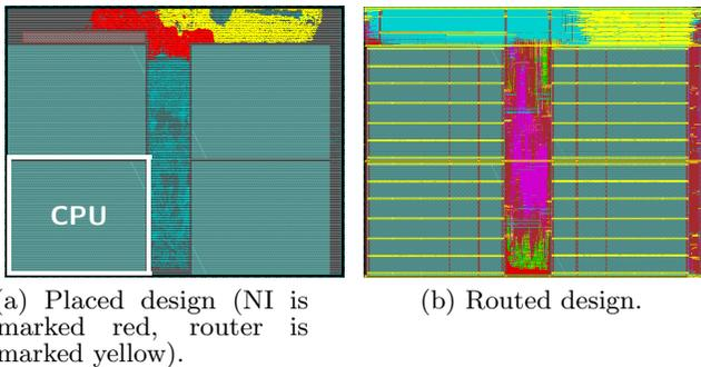
**Figure 6: Physical implementation of a CPU cluster with 4 CPU macros and 4 times 32 kB local memory. Area requirements are 0.70 mm<sup>2</sup>.**
