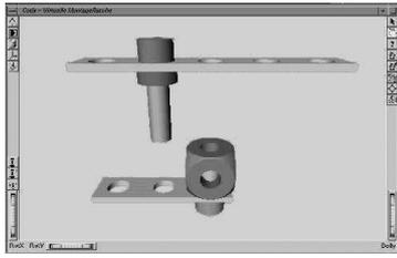
Figure 5: Original situation and first step of assembly example: The system is instructed: “Insert the aggregate into the bar”. The systems selects suitable objects and connection ports for the mating operation.
