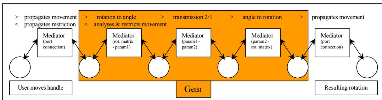
Fig. 8: A chain of CMs propagating a rotation action through a gear
