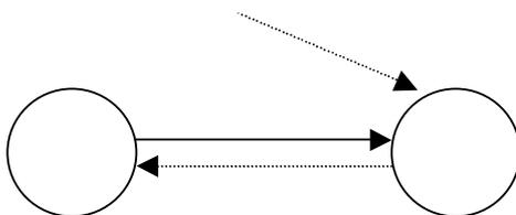
Fig. 2: A directed field connection, with forbidden connections (dotted arrows)
