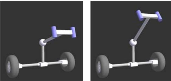
Fig. 10: Height adjustment of the steering wheel
