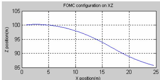
Fig 6. Vehicle dynamic simulation projection on  $E\xi\xi$  without FOMC
