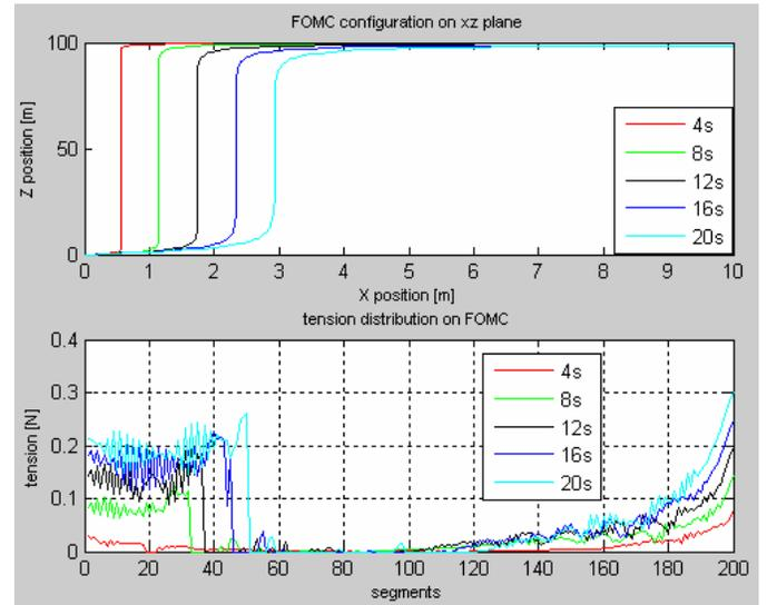
Fig 3. FOMC's tension distribution and shape with velocity of ocean current  $v = (0.15\text{m/s}, 0, 0)$
