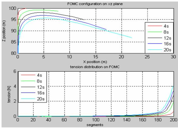
Fig 4. FOMC's tension distribution and shape under no ocean current
