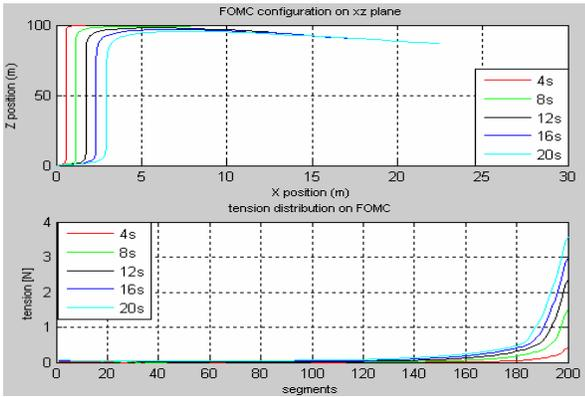
Fig 5. FOMC's tension distribution and shape under velocity of ocean current  $v = (0.15\text{m/s}, 0, 0)$
