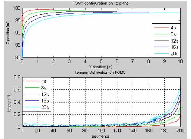
Fig 2. FOMC's tension distribution and shape with no ocean current
