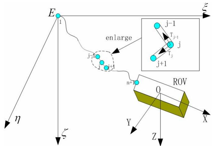
Fig.1:The inertial coordinate system and model of cable ROV(Remotely Operated Vehicle)
