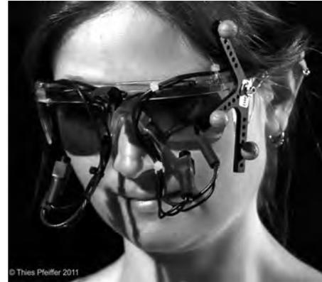
**Figure 1:** A head-mounted eye-tracking system by Arrington Research. It is augmented with an optical target for the DTrack2 tracking system by ART and with polarized filters for stereo presentations in a virtual environment. The modifications allow 3D gaze tracking in real and virtual environments.
