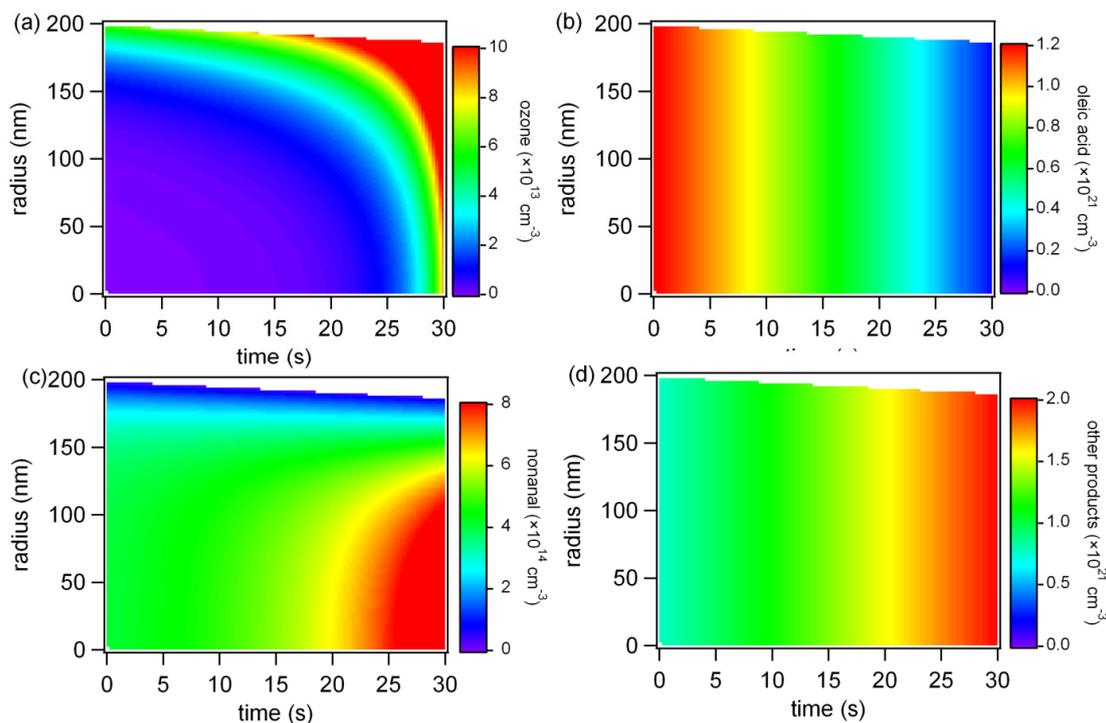
**Fig. 5.** Ozonolysis of oleic acid and evaporation of nonanal. Temporal evolution of bulk concentration profiles for (a) ozone, (b) oleic acid, (c) nonanal and (d) non-volatile products. The y-axis indicates the radial distance from the particle core to the near-surface bulk. The color shows the bulk concentration in units of  $\text{cm}^{-3}$  (blue = low, red = high).
