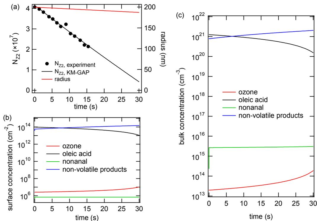
**Fig. 4.** Ozonolysis of oleic acid and evaporation of nonanal. **(a)** Experimental data (black symbols; Ziemann, 2005) and model results for the total number of oleic acid molecules ( $N_{Z_2}$ , black line) and for the particle radius (red line); **(b)** surface concentrations at the quasi-static surface layer and **(c)** average bulk concentration of ozone (red), oleic acid (black), nonanal (green), and non-volatile products (blue).
