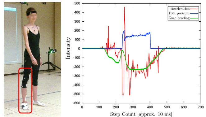
(a) Dancer equipped (b) Plot of a data sample recorded during a single jump with a BRIX stack.
