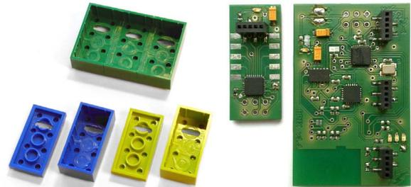
(a) Cases made of Lego bricks. (b) PCB of an extension module and a base module.
