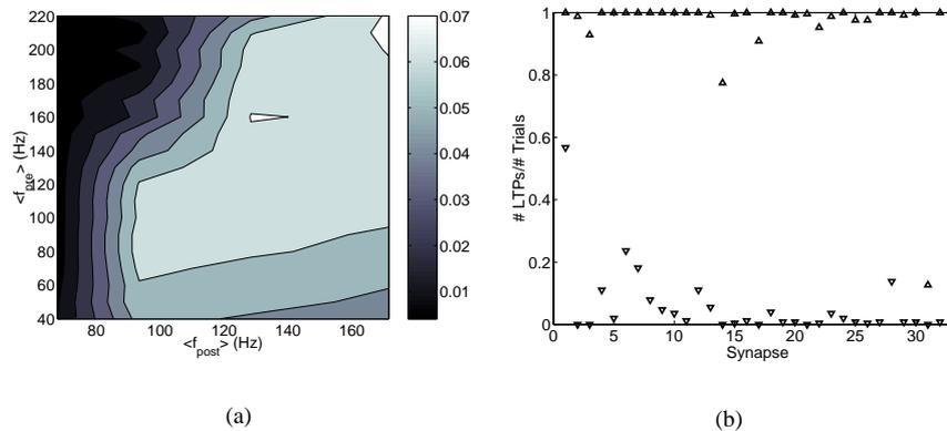
Figure 4: (a) CV of post-synaptic inter-spike interval (ISI) as a function of pre- and post-synaptic firing rates, measured for one plastic synapse. (b) Probability of inducing LTP measured over the whole row of synapses. Upward triangles correspond to the stimulation experiment that was expected to induce LTP while downward triangles correspond to the stimulation experiment that was expected to induce LTD (see text for details).
