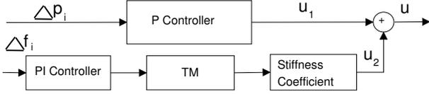
Fig. 5. Composite Position + Force Control Scheme.
