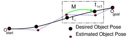
Fig. 1. Incremental manipulation of object pose  $O$ .
