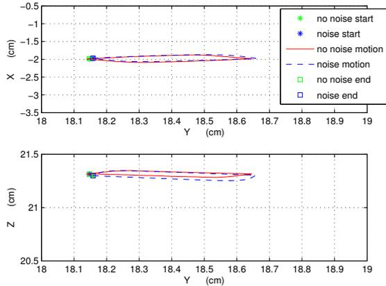
Fig. 7. Object motion parallel to contact normals ( $y$ -axis) as the ideal manipulation. Tracking error(maximum) is less than 20%. Multi simulation results, changing the controller parameters in Eq. 6 show that the composite controller parameters have the direct affection on the tracing error accuracy. A adaptive controller parameters regulation algorithm will be helpful in increasing the tracking accuracy comparing with this manual setting parameters.
