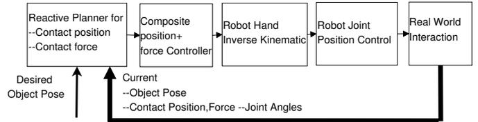
Fig. 2. Components of closed loop control scheme.
