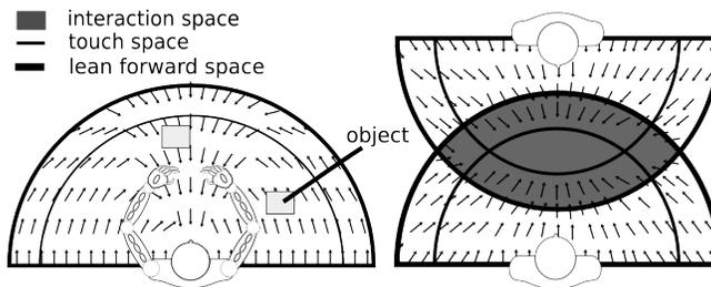
**Fig. 1.** Left: Subspaces surrounding a virtual human. Lean-forward space as an extension of touch space. Arrows illustrate force vectors in a repulsive artificial potential field, here pointing to the front of the body. Right: Interaction space spanned by two partners.
