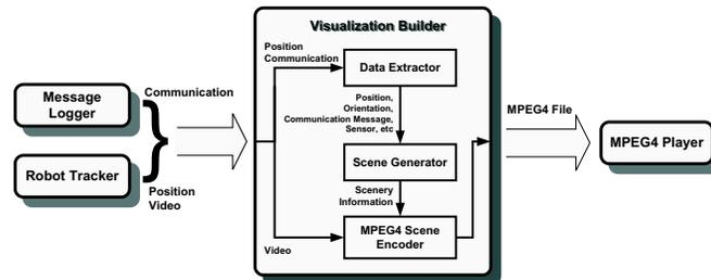
Fig. 2. The process flow of the visualization generator.
