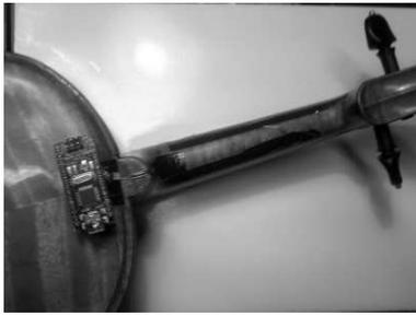
**Figure 3:** Picture of the violin mounted pressure sensors.
