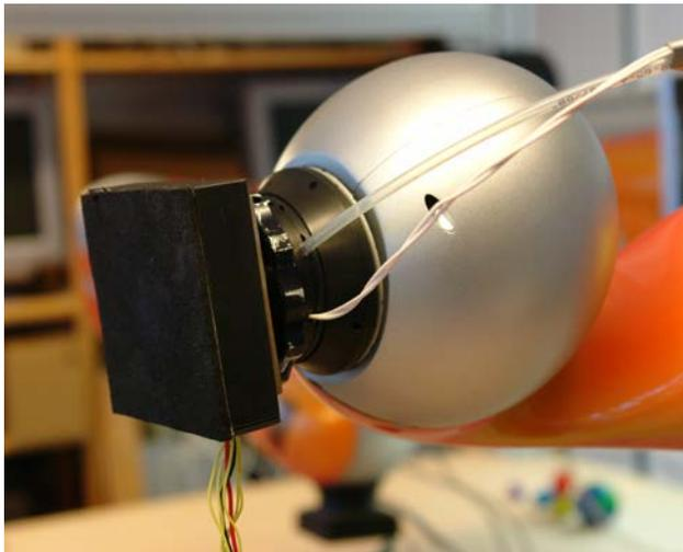
**Figure 2:** The myrmex sensor mounted on the Kuka LWR end effector. The internal cabling (air and power) that can be seen in the picture are not used in this setup
