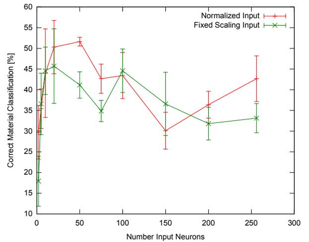
**Figure 10:** In this graph the correct classifications of the material surface texture are plotted. In this even for humans difficult task, a good generalization could not be achieved.
