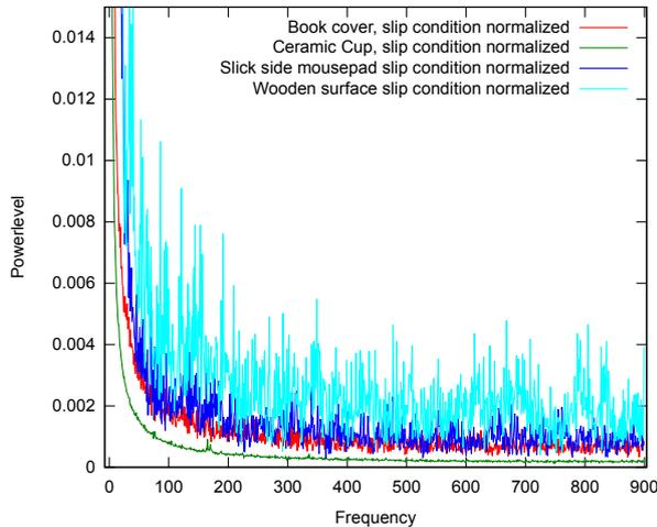
**Figure 6:** In this graph, the averaged and normalized frequency spectra of different surfaces are exemplary shown. To enhance the readability only four of the five different materials are displayed.
