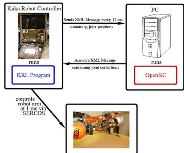
**Figure 3:** Control Scheme of the Kuka LWR using the RSI XML interface. The XML messages are send over Ethernet and allow real time controll over the Kuka Robot
