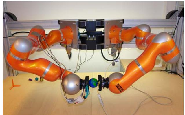
**Figure 1:** The bi-manual setup in the tactile lab. Both Kuka LWRs have a myrmex tactile sensor mounted on their end effectors. Both sensors have magnetic connectors which act as predetermined breaking points in case of accidentally high contact forces.
