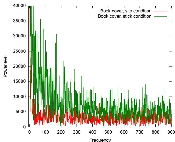
**Figure 5:** The graph shows the spectrum of two samples. Both samples come from the same experiment. The sampled object is the book cover. A clear distinction between a slip and stick condition can be made.
