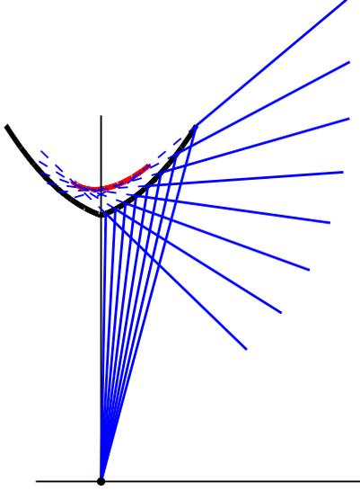
Fig. 2. The viewpoints of a reflective surface with constant elevational gain lie on a caustic surface (red curve) defined in (4). All principal rays are tangent to the caustic.
