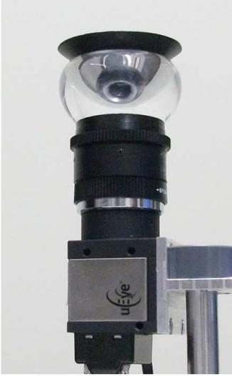
Fig. 6. Picture of the first prototype of an omnidirectional imaging system with constant elevational gain and single viewpoint. Diameter of the transparent globe is 48 mm.
