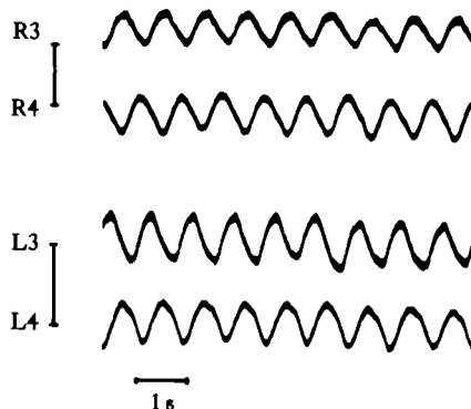
Fig. 1. An example of a record of four legs. Return stroke movement is upwards. L, left; R, right legs; legs are numbered from front to rear. Left and right legs were recorded with different gain; vertical bars indicate  $5\text{ cm}$ . Treadmill speed,  $11\text{ cm s}^{-1}$ ; load,  $0\text{ g}$ .
