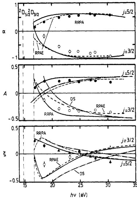
**Figure 3.** Photoionisation of Hg 5d. Experimental results for the spin parameters  $\alpha$ ,  $A$  and  $\xi$  for the final ionic state  $^2D_{5/2}$  (full symbols) and  $^2D_{3/2}$  (open symbols). Triangles (for  $\xi$ ), Schönense *et al* (1982); full curves, RRPA calculation of Johnson *et al* (1982); broken curves, RPAE calculation of Ivanov *et al* (1979); chain curve, DS calculation of Keller and Combet-Farnoux (1985). The vertical broken lines indicate the ionisation thresholds.
