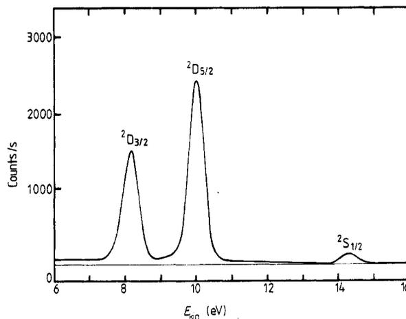
**Figure 1.** Photoelectron spectrum of Hg ( $5d^{10}6s^2$ ) recorded with a monitor channeltron behind the spectrometer using circularly polarised light of 50 nm wavelength. The final ionic states are indicated.
