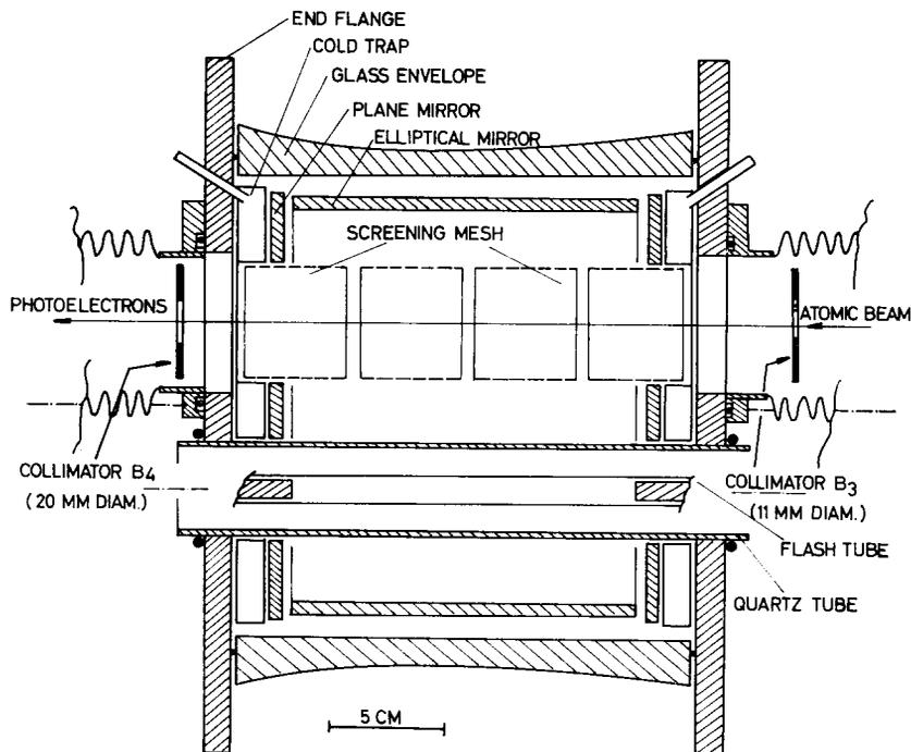
Fig. 3. Longitudinal section of the ionization region.
