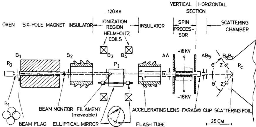
Fig. 1. Sectional view of the whole apparatus, semi schematic (details near the axis not to scale); A: Deflecting plates;  $B_n$ : Collimators; Z: Electron detector; Pressure in the vacuum tanks:  $p_0 = 5 \times 10^{-6}$ ,  $p_1 = 2 \times 10^{-6}$ ,  $p_c = 5 \times 10^{-6}$  Torr.
