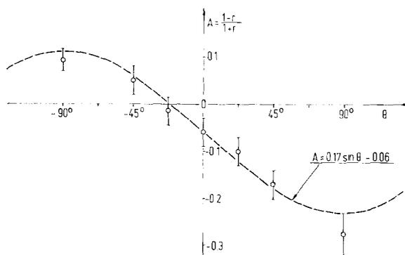
Fig. 4. Polarization asymmetry  $A$  recorded by transferring the electron spin direction in steps from  $+90^\circ$  (up) to  $-90^\circ$  (down).
