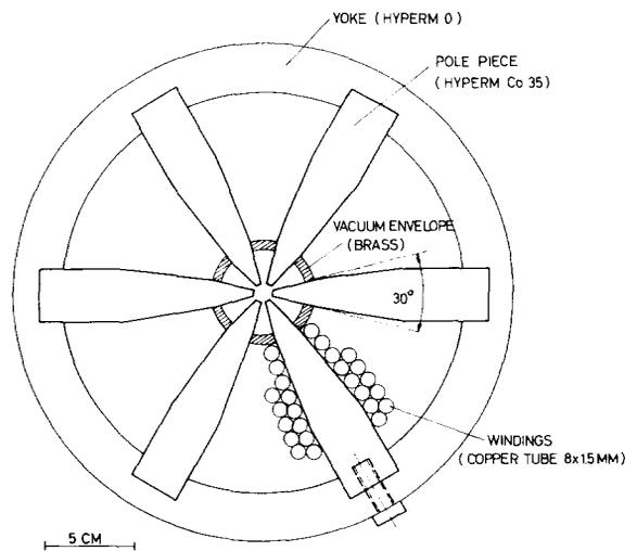
Fig. 2. Cross section of the six-pole magnet.
