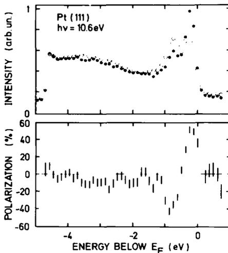
Fig. 1. Spin-resolved photoelectron spectrum of Pt(111) for normal incidence and normal emission at 300 K. Upper part: Intensities measured with the two counters in the Mott detector, solid and open circles. Lower part: Corresponding electron-spin polarization obtained from the data in the upper part and normalized to a complete circular polarization of the light. The experimental energy resolution  $\Delta E$  is 150 meV FWHM (improved with respect to ref. [3]).
