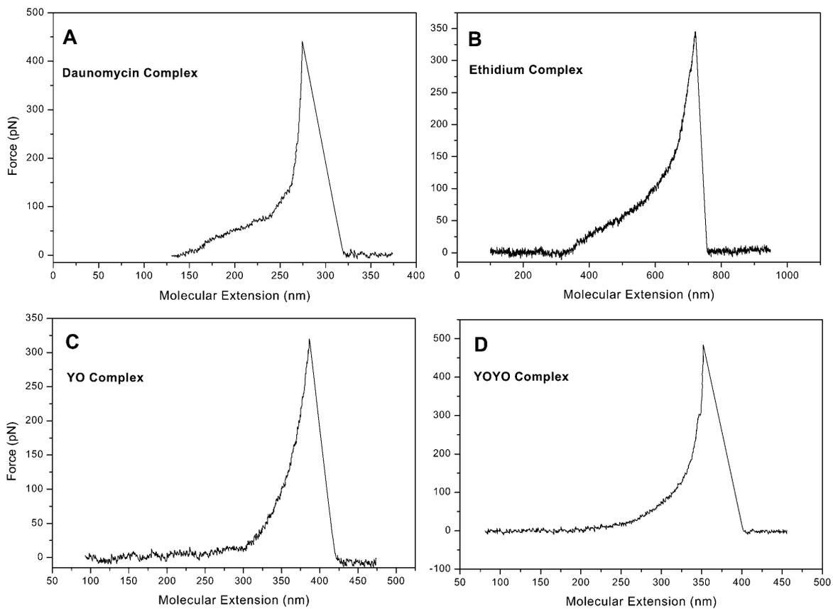
FIGURE 3 Force-extension traces for the complexes of poly(dG-dC) dsDNA with the intercalants (A) daunomycin; (B) ethidium bromide; (C) YO; (D) YOYO.
